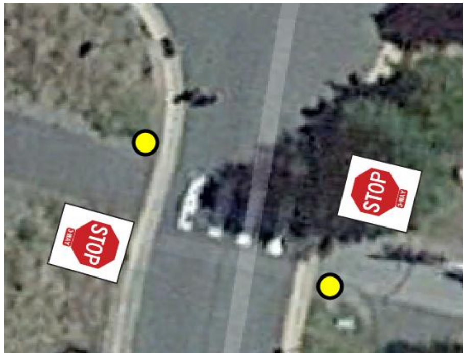
Existing Lakefront Path crossing with STOP signs for cyclists and flexible bollards placed across from STOP signs
