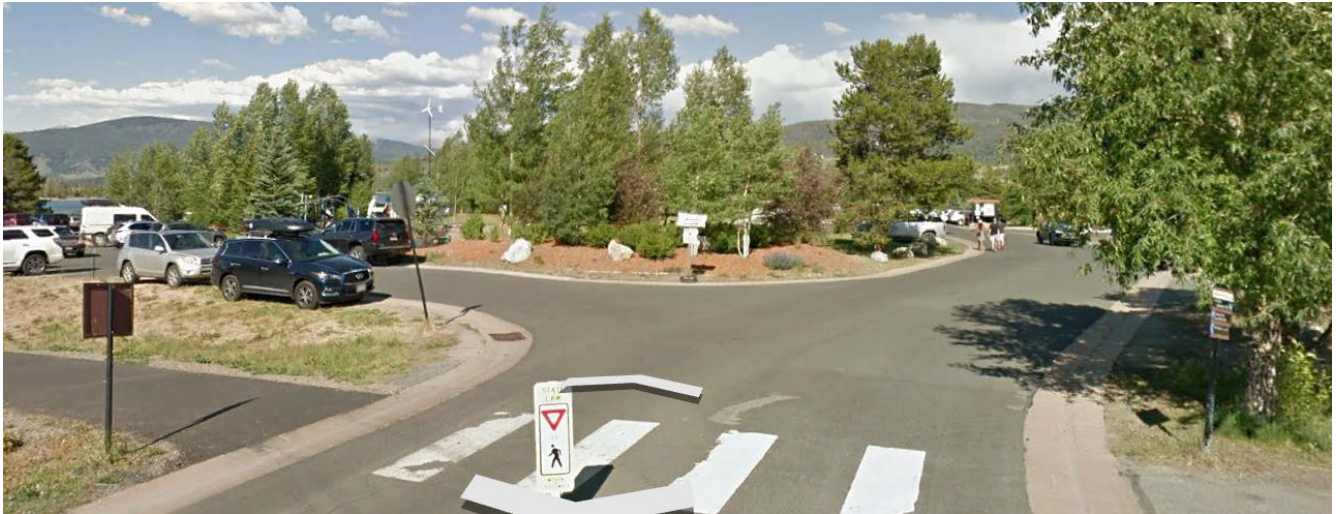
Existing single crossing for reservoir recreation path, showing no continuing sidewalk as well as trees and vegetation obstructing view of park for approaching pedestrians
